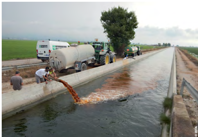
Pilot test of injection of sediment into the Ebro Delta irrigation network.
